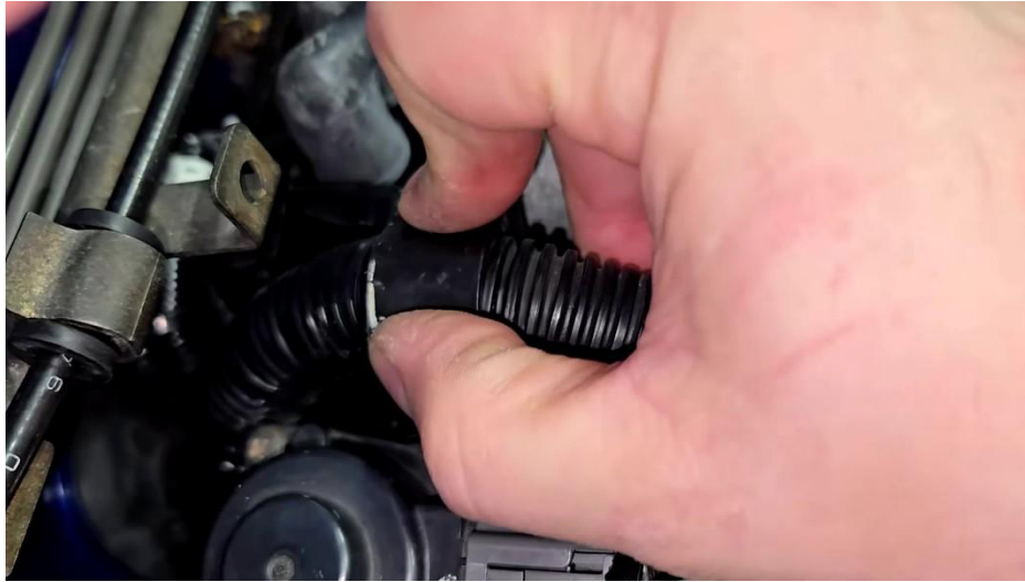
Figure 16. Front harness clamp shifted rearward for connector slack.
