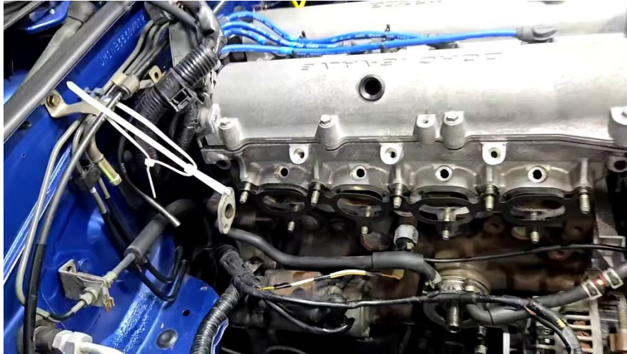
Figure 5. EGR crossover tube supported above the manifold opening.
