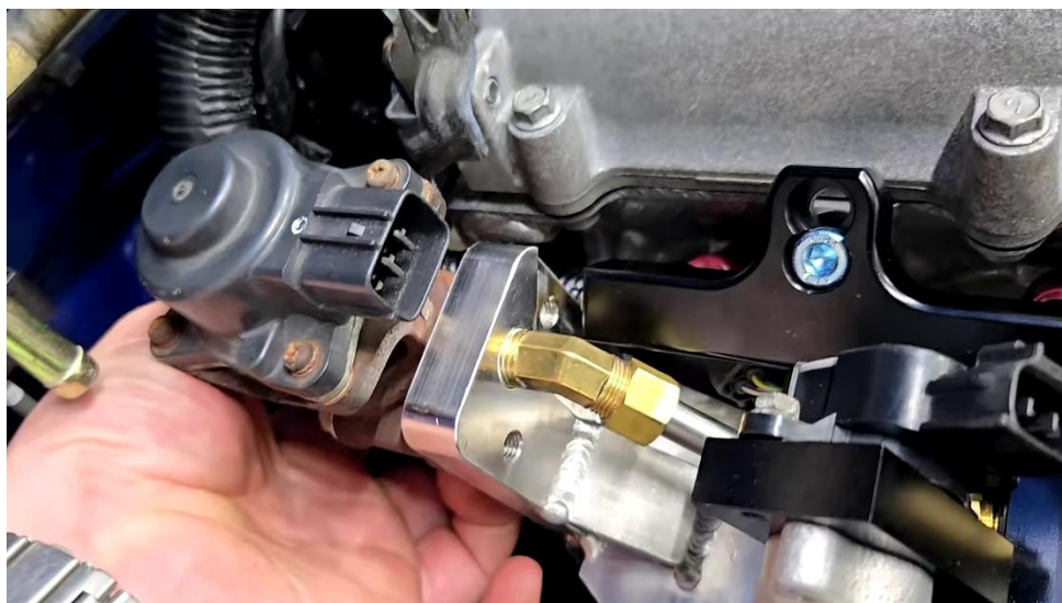
Figure 19. EGR valve installed with the upper solenoid rotated for fuel-rail clearance.
