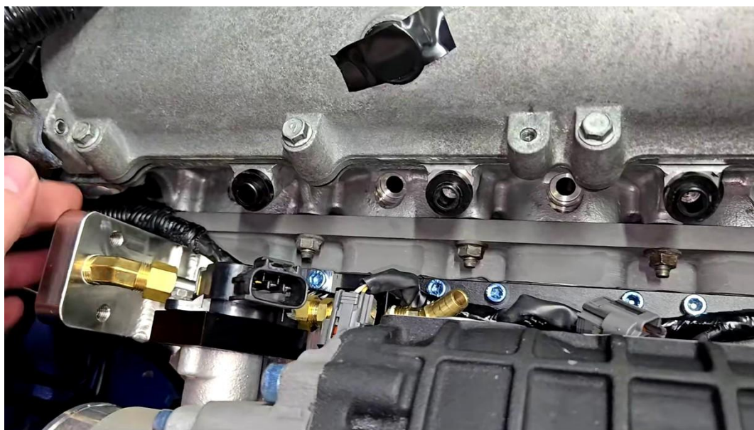
Figure 15. Completed engine-harness routing above the supercharger/manifold assembly.
