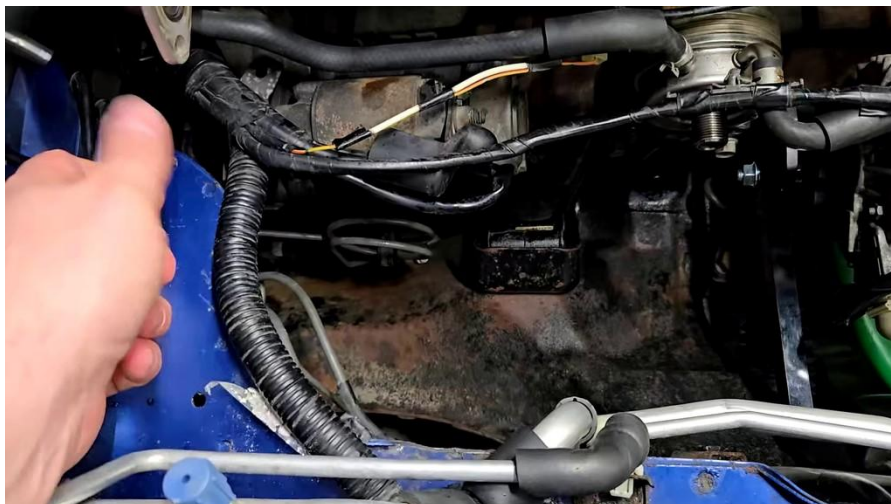
Figure 4. Starter-side harness repositioned into the engine-bay ledge.
