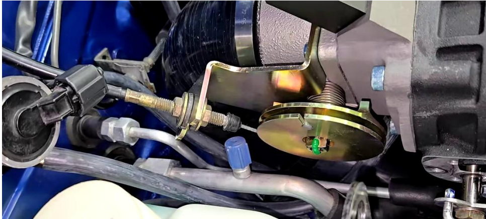
Figure 31. Throttle-cable routing at the guide pulley and throttle arm.
