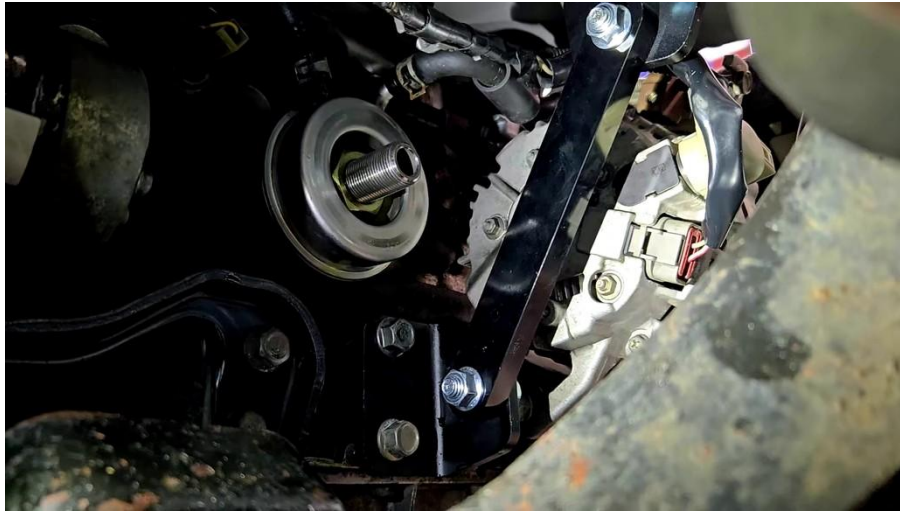
Figure 9. Completed underbrace installation viewed from below.
