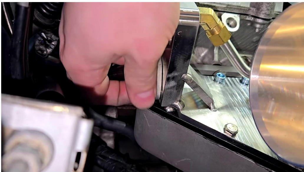
Figure 10. EGR crossover-tube connection at the FFS manifold bracket.
