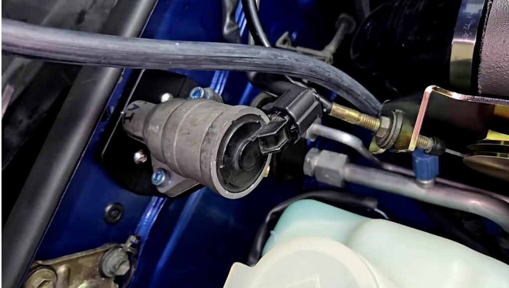
Figure 20. IAC Valve and supplied bracket installed on the driver-side firewall.
