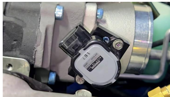
B - TPS installed
