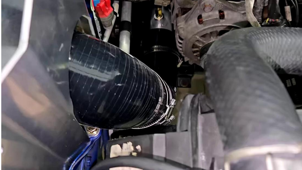
Figure 24. MAF-side silicone coupler adjusted for alternator, fan and chassis clearance.
