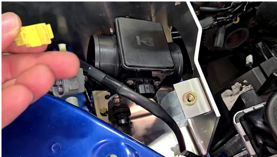
Figure 22. Yellow MAF-connector secondary lock removed for connector passage into the airbox.
