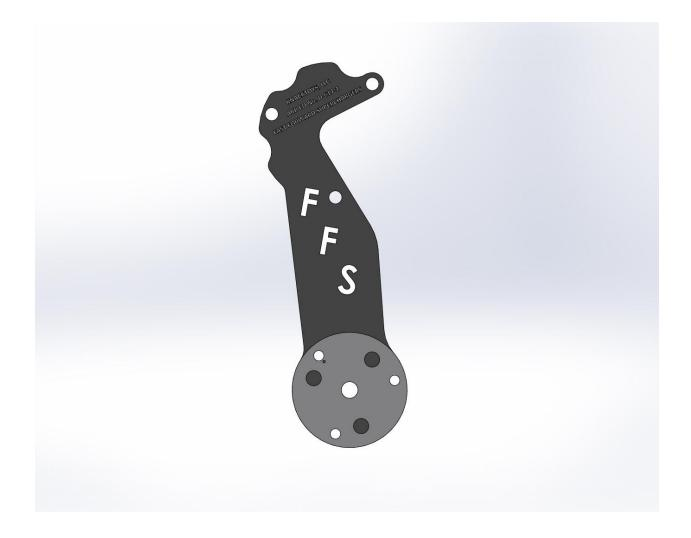
Note that the threaded hole and the associated large hole are closer together. This will cause the tensioner to rotate down slightly at the belt and make a little more room. For those who venture beyond 130mm to 140mm or 150mm or larger, you can flip the spacer over and get three more choices to make up for the lower belt return position. For those of you with older kits and now starting to add a lot more power, this applies all the way back to the first kit shipped in 2005.
