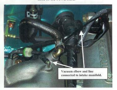
3. If your Miata doesn't have a vacant vacuum fitting then disregard the elbow, you will need to T into an already used fitting. Locate an appropriate vacuum fitting on the intake manifold preferable on the top towards the firewall. Pull off the vacuum hose currently attached to it. Cut a 2" piece
