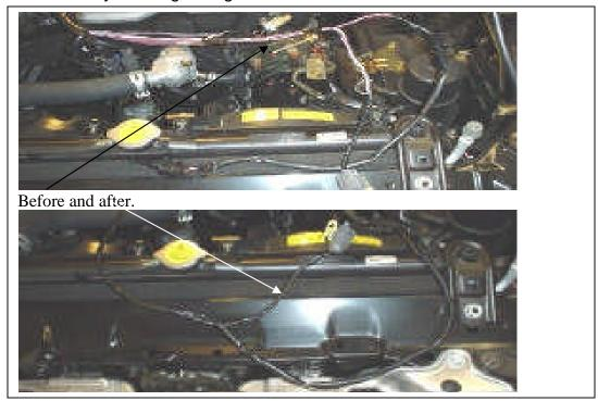
12) Remove the 12mm bolt holding the wiring harness bracket at the back of the engine. Then flip the wiring harness bracket and attach as shown. Zip tie the wiring harness as shown. This is to ensure adequate clearance from the EGR.
