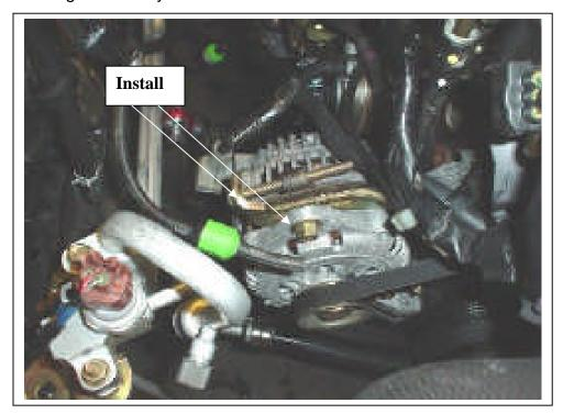
16) Install the alternator belt and tension by tightening the 12mm alternator tension bolt. Then tighten the 12mm alternator tension hold bolt and the 14mm alternator pivot bolt.
