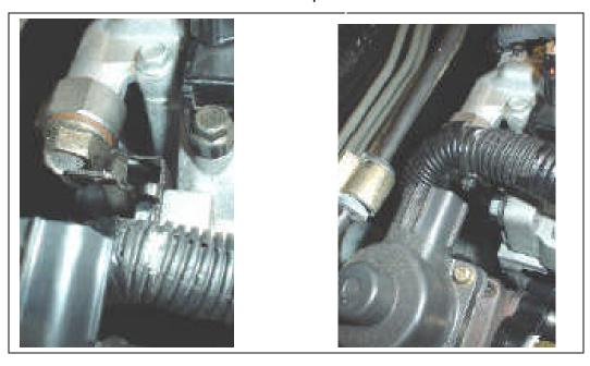
13) Bolt up the brace to the supercharger intake manifold with the 14mm bolts and nut. Do not install the brace to the engine block yet.
