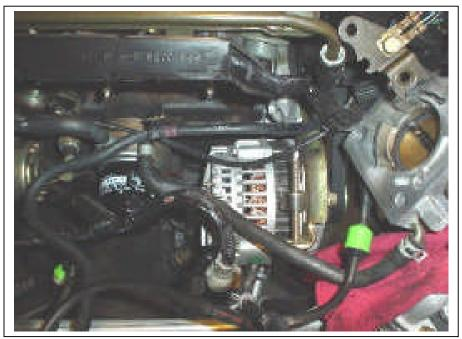
34) Unclamp the hose on thermostat side going from throttle body and remove. Put the two removed clamps and rubber sleeve on the replacement coolant hose. Attach the replacement coolant hose to the thermostat barb and zip tie the rubber sleeve as shown to protect the coolant hose from the alternator bracket.
