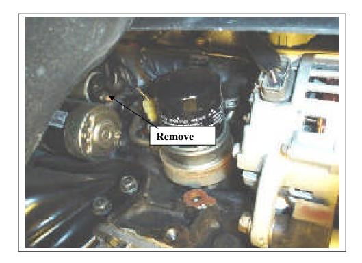
32) Tilt the intake manifold up and remove the 10mm bolt holding the fuel hose under the intake manifold.
