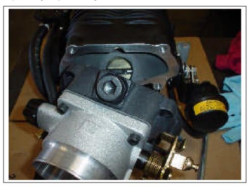
5) Apply a thin film of ultra black to the perimeter surface of the intake manifold and install the supercharger on the manifold. Replace the perimeter bolts.
