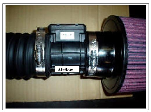
21) Position the filter as shown, and then connect the wiring plug to the MAF.
