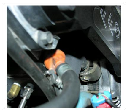
42) Connect the fuel rail to the original fuel line. The preferred method is to connect the fuel line to the rear of the fuel rail with the FPR on the front end of the fuel rail and a pipe plug in the top fitting.
