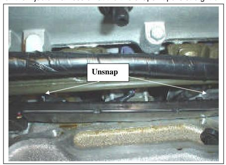
26) Remove the injector harness cover and remove the tape from the wires. Carefully unplug the harness from the four injectors making note of which plug goes to which injector. Then re-tape the harness (without the cover) and attach it above the fuel rail with zip ties as shown. Connect the four electrical connectors back to the four injectors.
