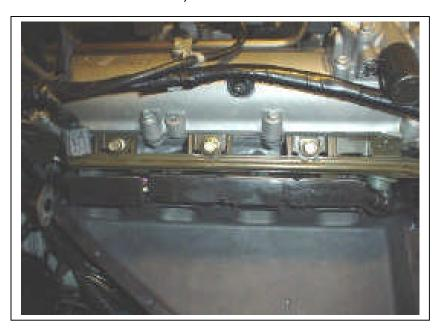
2) Install the fuel injectors and the new fuel rail. Replace the bolts.
