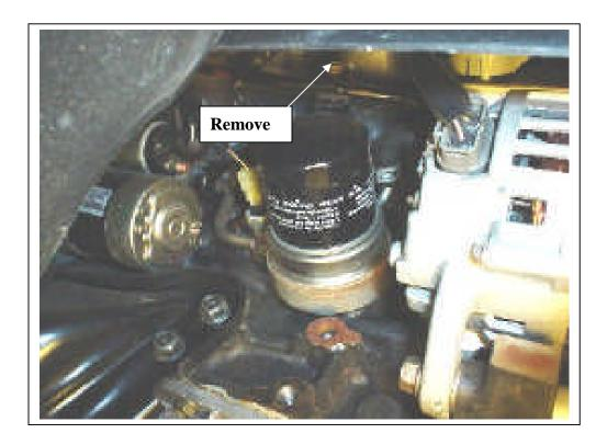
31) Remove the 10mm bolt holding the oil line under the intake manifold. It is behind the fuel hose in the picture.
