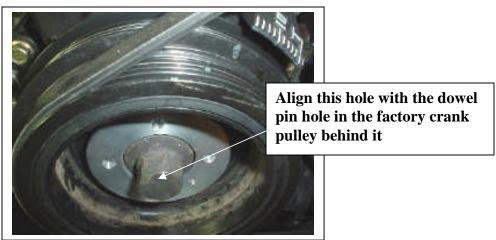
30) Install the supercharger crank pulley with the included four 10mm bolts that are longer than the originals. Be sure to line up the hole on the crank spacer with the hole in the supercharger crank pulley. (Note: Do **NOT** use Loc-Tite on these bolts)
