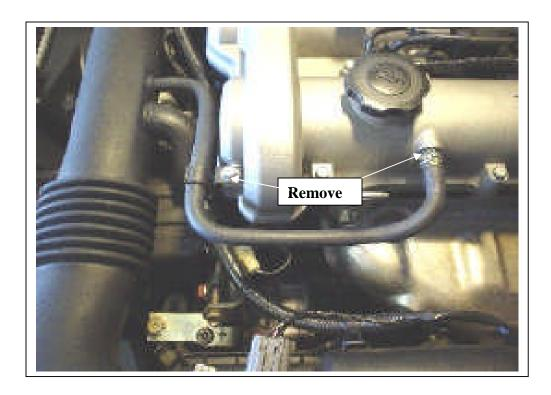
6) Loosen the crossover tube clamps and remove the crossover tube.
