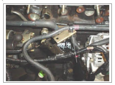
36) Remove the clamp from the wiring harness as shown.
