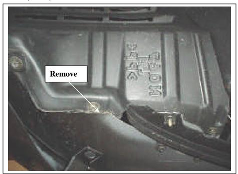
29) Remove the lower 14mm bolt from intake manifold support brace and remove the support brace.
