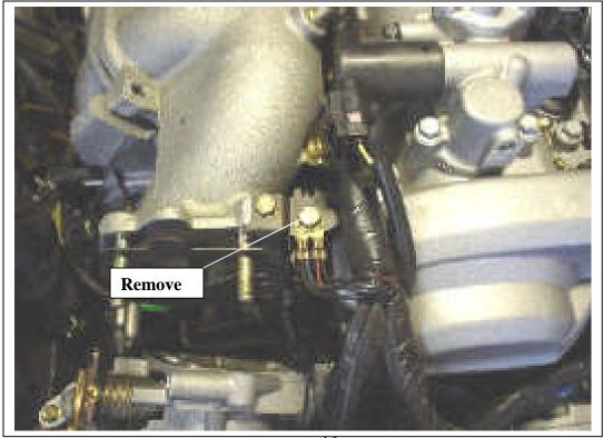
20) Remove the short hose connecting the upper and lower intake manifold.
