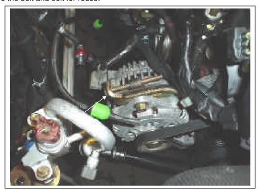
40) Remove the 12mm alternator tension hold bolt. Save the bolt for reuse.
