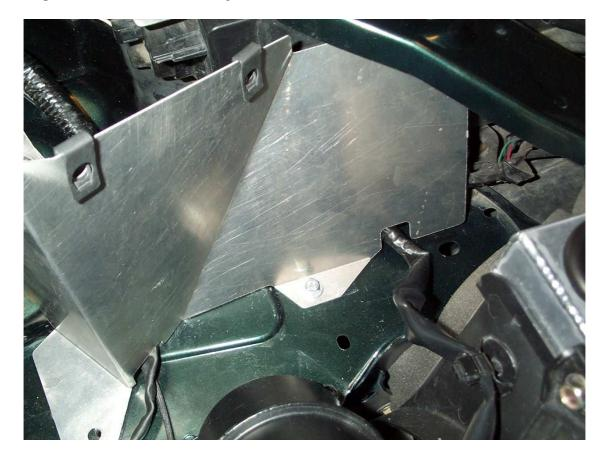
Step 5. Fasten the front mounting bolt and leave loose.
