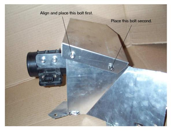
Step 14. Fasten rear screw on passenger side of lid then the front screw.
