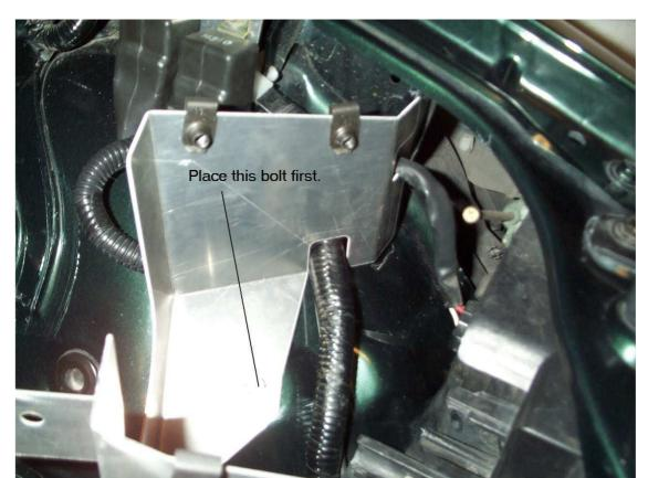
Step 4. Place the air box base and route the wires along the air box cutouts and fasten the mounting bolt inside the box. Do not tighten the bolt.
