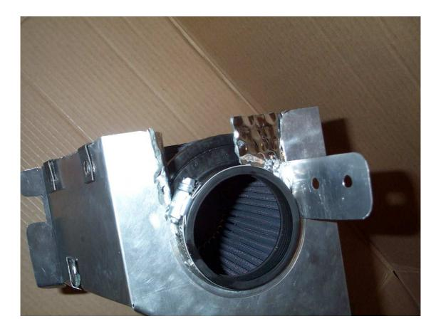
Step 11. Place MAF into filter flange and line up with mounting holes and mount to box then tighten the filter clamp to secure filter to the MAF.
