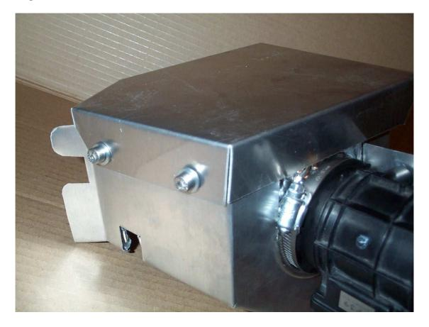
Step 13. Fasten both screws driver's side of lid and leave loose.
